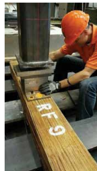
» A bamboo rail tie produced by Resource Fiber undergoes testing in a lab. Photo credit: Resource Fiber
