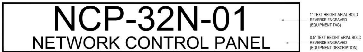
PRIMARY NAMEPLATE: 2-LINE 2-INCH HIGH LAMACOID LABEL c/w ADHESIVE BACKING
