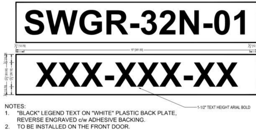
Figure 2: Example of Distribution Panel Primary Nameplate
